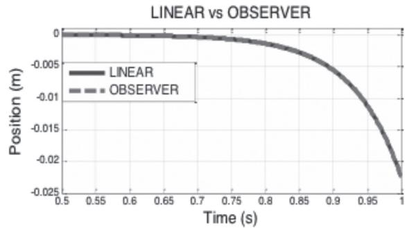
**Figure 9.** Comparison of the output of the nonlinear model with the observer in open loop.
