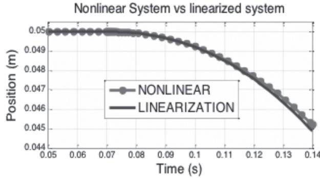
**Figure 4.** Nonlinear model vs linearized model with respect to the second variable of state.
