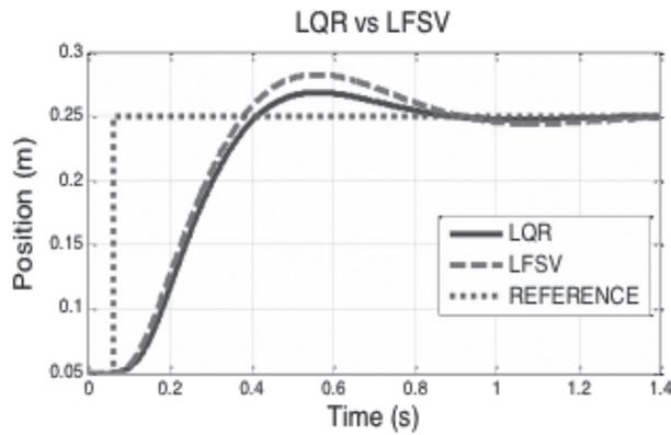
Unlike the previous result presented in figure 14, where there is a outcome in favor for the controlled system with the LQR. In figure 15 the linear system is not a significant difference between the behavior of the system compared by the drivers and LFSV LQR, it should be noted that the non-linear system is more closer to the actual behavior of the system.
