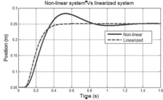
The initial undershoot observed, refers to the control effort required to place the ball in the equilibrium position (figures 7 and 11). Control action used for LFSV, both from linear and non linear systems, is presented. As can be observed, the nonlinear system has a greater over-impulse than the linear one (figure 7).
