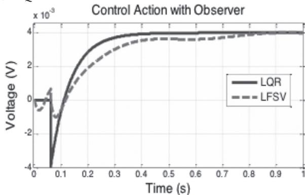
In this way, the results for the non-linear system, when you enter a measurement noise variance of  $1 \times 10^{-15}$ , where it is possible to verify the behavior of the system with regard to its position. In figure 20, this noise is negligible for the LQR controller, but you can observe a large variability in the response of the driver RLVE, which dramatically affects its stability.
