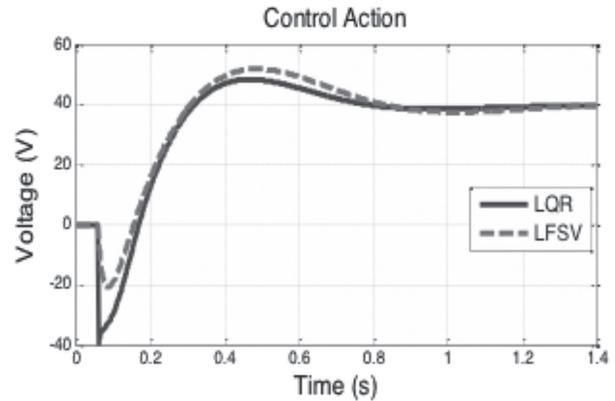
The result obtained in figure 17, presents a similar behavior in the sub-impulse as explained in the figure 16, although it does not feature an on momentum as evidenced in the above figure, such behavior exposes that the sub-impulse is present in the linear model and non-linear without the driver, therefore it is a behavior of the system itself.
