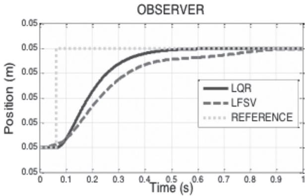
With respect to the control action that is presented in figure 19, the non-linear system with observer responds faster before the sub-impulse, with a time less than 0.1 seconds, and with an energy expenditure 10 times less than the submitted to the same system without observer. In this way, the system with observer presents a better behavior before the sub-impulse.
