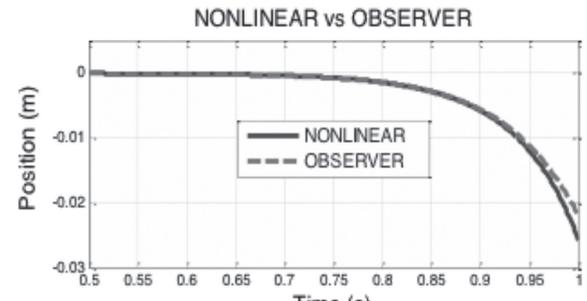
It compares the observer with LFSV for both linear and nonlinear systems. For the former, it can be observed that the response is similar to the LFSV without observer. For the nonlinear, greater error and establishing time can be seen. Nevertheless, the observer is considered to be suitable for the magnetic levitator (figure 10).
