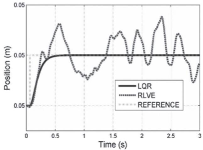
**Figure 21.** Control action of the non-linear system with observer in a noise measurement.
