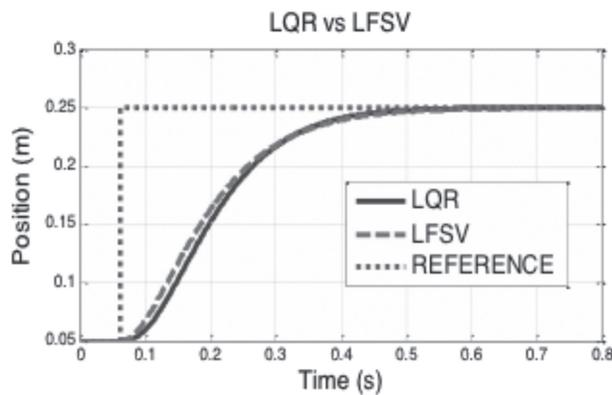
In figure 16 you can see a sub-impulse, before spending the 0.2 seconds, in which the sub-impulse of greater magnitude and presents the system controlled by LQR, this is reflected in a higher cost of energy, that's costing you more to the controller, but is subsequently offset with the on momentum between the (0.4 to 0.6) seconds less pronounced in front of the driver LFSV.
