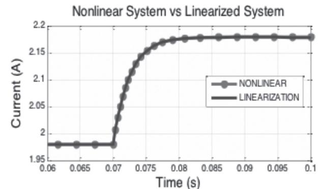
In conclusion, with respect to linearization, it can be observed that in the three figures shown above (figures 3, 4 and 5) the linear model follows the nonlinear one for small changes in input. For this reason, linearization is the right choice and it represents the nonlinear model correctly.
