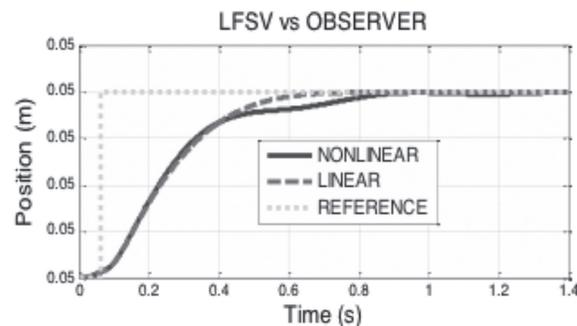
Control action of LFSV, with and without observer, in which it can be seen that both signals are very similar.
