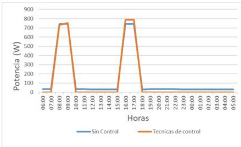
Figura 10. Comparativo consumo diario potencia consumida acometida, Sin Control Vs Técnicas Figure 10. Comparative daily power consumption, without control vs. techniques
