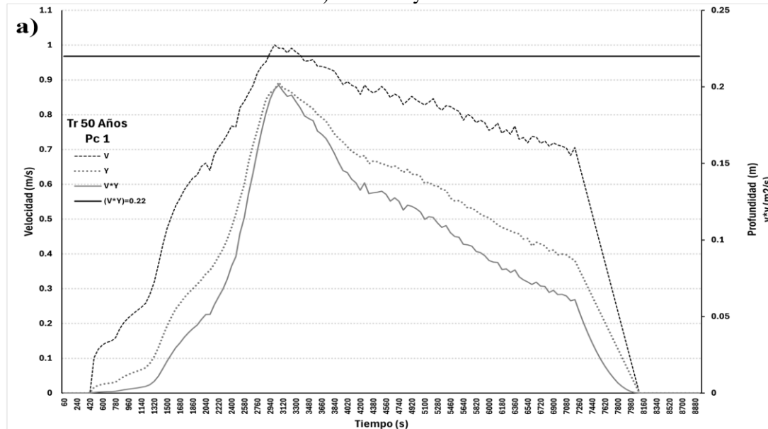
Figure 4. Evolution of Velocity ( v ), Depth ( y ) and Product ( v*y ) over time for Pc1: a) Tr = 50 years and b) Tr = 100 years.
