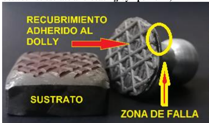
Figura 5. Falla adhesiva entre sustrato y recubrimiento por "pull off". (Adhesive failure between substrate and coating by "pull off")
