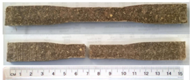
Figure 1. Composite probes obtained for tensile strength tests according to standard ASTM D638-10.
